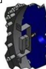
CONTRAST SCREW FOR THE SENSOR OF "FLANGE HORIZONTALITY" ASSEMBLED ON MASTER FLANGE
